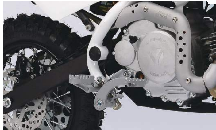
PROTECTION MAITRE CYLINDRE FREIN ARRIÈRE (POUR PILOT/ FACTORY SAUF 2016) REAR BRAKE MASTER CYLINDER GUARD (FOR PILOT/ FACTORY EXCEPT 2016)
